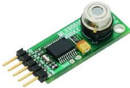
MLX90614 Infrared Thermometer Module
